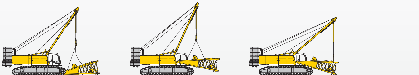
Unloading and assembly of boom foot
