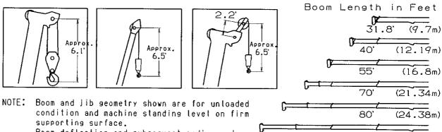
Boom deflection and subsequent radius and boom angle change must be accounted for when applying load to hook.
