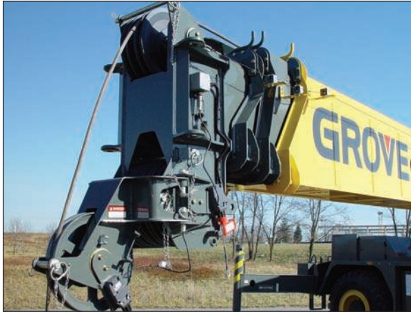
The RT540E incorporates a rectangular boom shape made from 100k.s.i. steel which eliminates weight and maximizes structural capacities.
